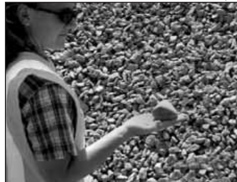
Recycled concrete aggregate piled at the Lafrate Crushing Plant in Taylor, Michigan.
