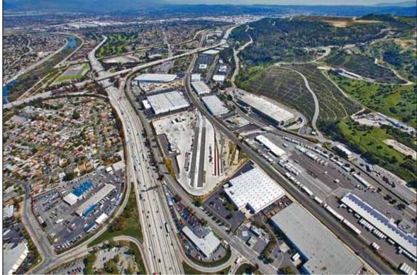
This aerial view shows the Puente Hills Intermodal Facility, materials recovery facility and landfill complex (from left to right) located in Los Angeles County, California. The intermodal facility and materials recovery facility are key components of the Sanitation Districts of Los Angeles County's waste-by-rail system.
