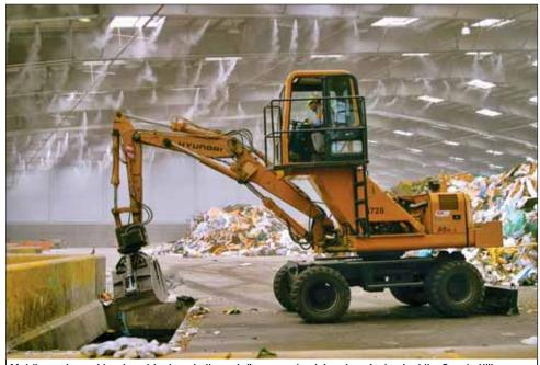
Mobile equipment loads residual waste through floor opening into a transfer truck at the Puente Hills materials recovery facility.
