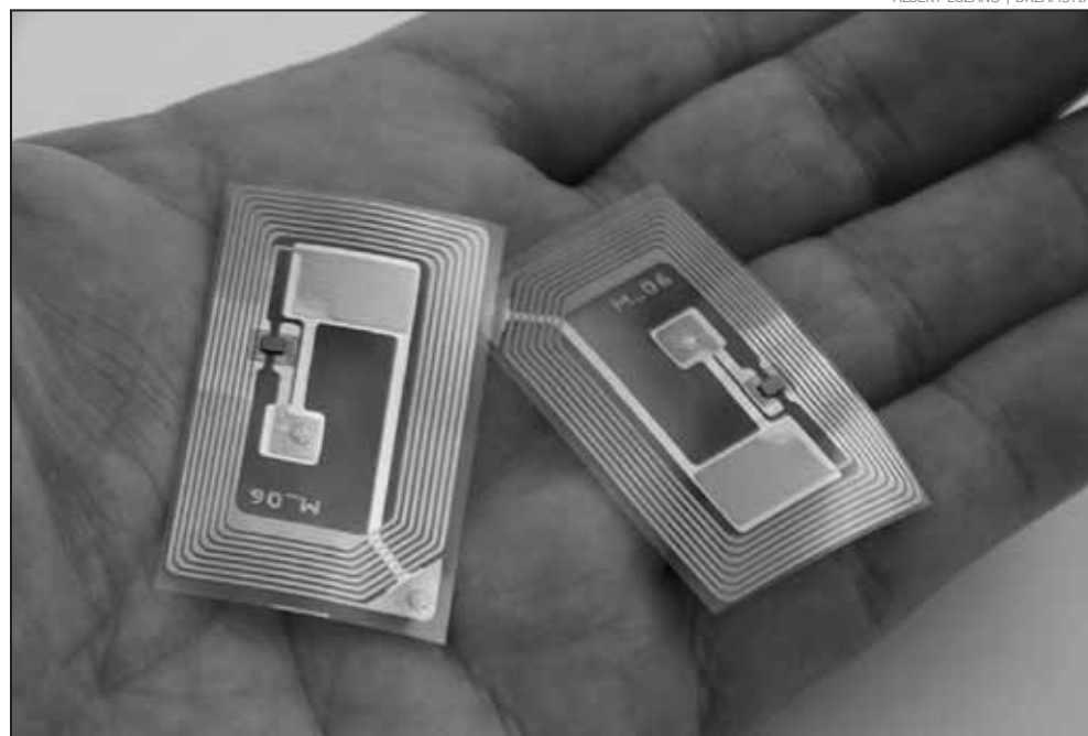
Radio frequency identification (RFID) tags are employed throughout the United States to track waste output and encourage recycling.
