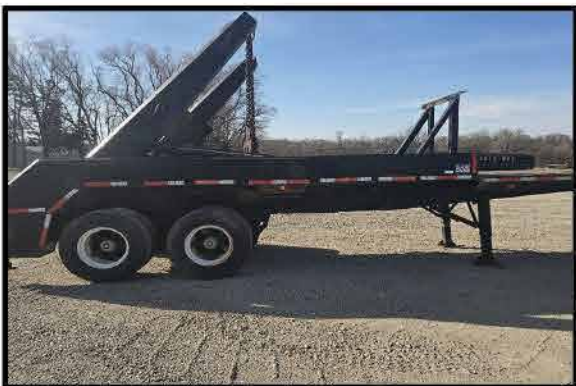
2003 ACE TRUCK BODY CO LUGGER BODY LUGGER BODY HAS 50,000 LB CAPACITY AND 120' ARMS
