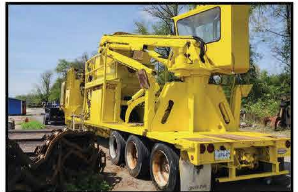
1989 SSI PORTABLE HOOK SHEAR SHREDDER 430HP MOTOR. DUAL SHAFT. 45"X75" CHAMBER.
