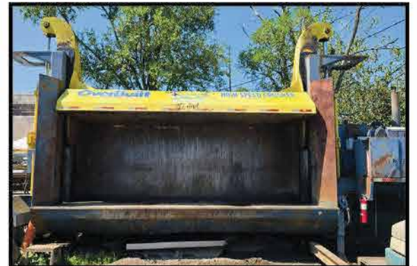
2001 OVERBUILT MODEL 10HS AUTO CRUSHER CRUSHER OPENING 20'3" WIDE, 10' HIGH WHILE OPEN
