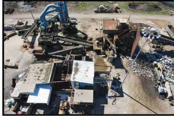
SVEDALA 98X108 HAMMERMILL AUTO SHREDDER FERROUS AND NONFERROUS DOWNSTREAM, 96"X115" INFEED
