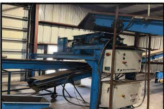
BUNTING MAGNETIC DRUM SEPARATOR 12' DIAMETER X 16' EFFECTIVE WIDTH NEODYMIUM DRUM
