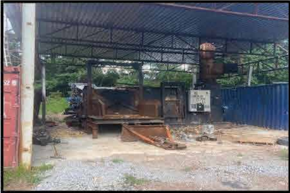
US FURNANCES MAX-4000 ALUMINUM SWEAT FUR. NEW BURNERS, 4,000 LBS HOLDING WELL, DATA LOGGER
