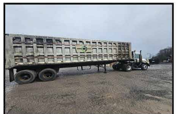
1994 JB-TL 36 FOOT END DUMP TRAILER 36 FOOT TRAILER, 87 INCHES DEEP, 90 INCHES WIDE, TANDEM AXLE
