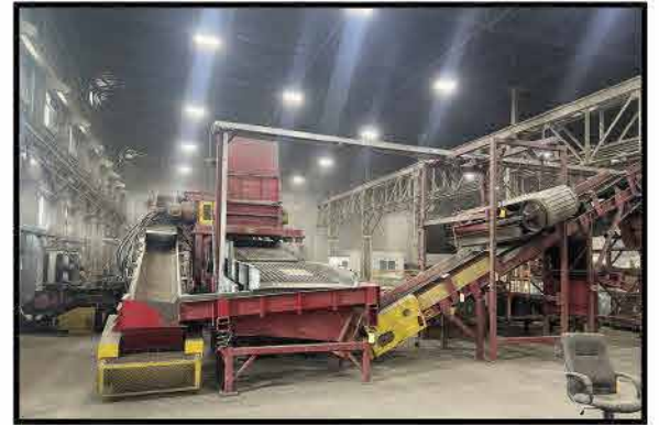
IDM RAPTOR COMPLETE SHREDDING LINE TWO DUAL SHAFT SHREDDERS, CONVEYANCE, EDDY, MAGNETS!
