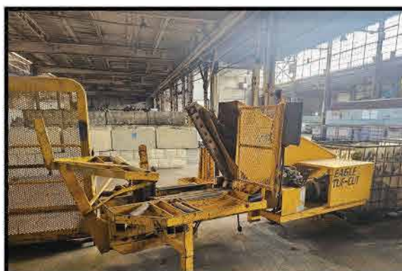
EAGLE TUF-CUT TIRE CUTTER STATIONARY MODEL, PROCESSES CAR, TRUCK AND MIXED OTR TIRES
