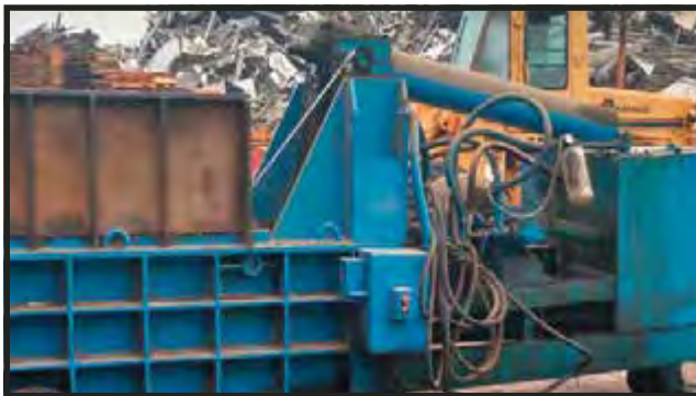
Mosley Portable Tin Baler 24" x 32" bales. 40 HP motor.
