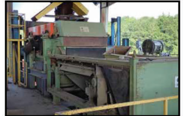
SGM 60" EDDY CURRENT WITH DSRP 2007 MODEL VIS 244 100/250. INCLUDES VIBRATORY INFEED!
