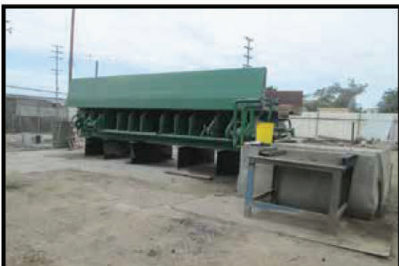
MOSLEY 330T 300 TON SHEAR AND SIZER WAS IN OPERATING CONDITION WHEN TAKEN OUT OF SERVICE
