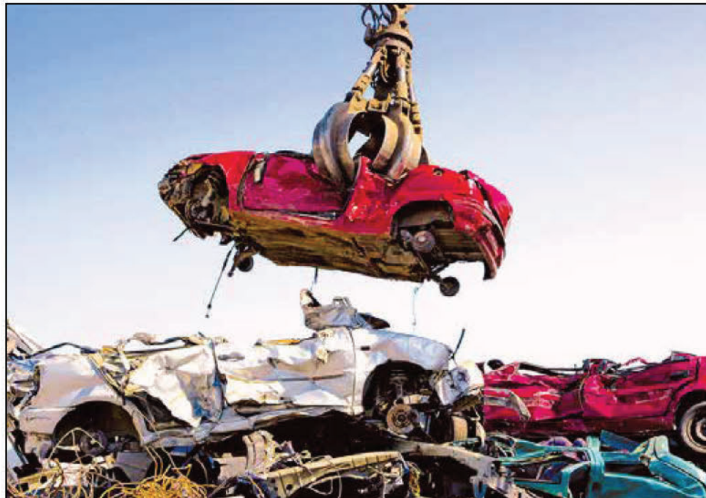
End-of-life vehicles are filled with flammable liquids, which could result in serious injuries to workers.
