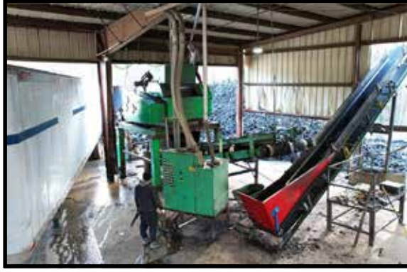
CM MULTI-STACK TIRE SHREDDER AND CONVEYORS ROTOR WAS REBUILT WITH NEW KNIVES AND SEATS REPAIRED!
