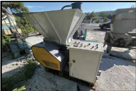
CABLE MANAGEMENT WIRE CHOPPING SYSTEM INCLUDES SHREDDER, GRANULATOR, AND AIR SEPARATION SYSTEM!
