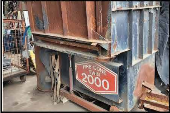
FIRE CONE TWIN 2000 ALUMINUM SWEAT FURNACE HAS AN AFTERBURNER. 1.5M BTUS
