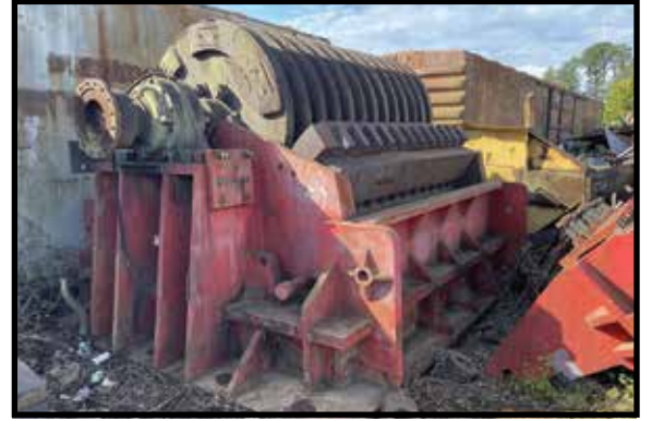
NEWELL 80X104 HAMMERMILL SHREDDER TOP FEED, BOTTOM DISCHARGE. LIKE NEW LINERS, GRATES, ROTOR.
