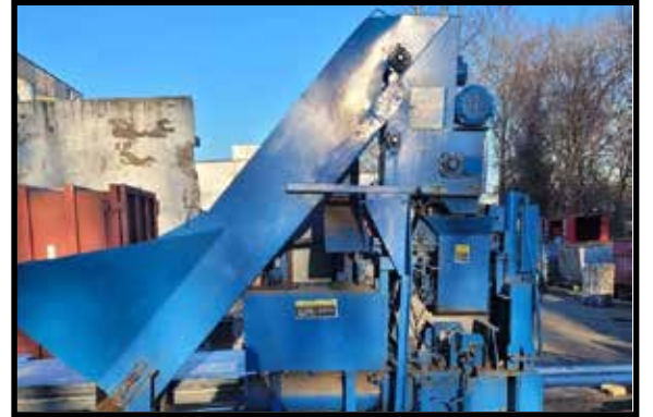
MOSLEY ALUMINUM CAN DENSIFIER INCLUDES CONVEYOR WITH HOPPER AND CONTROLS
