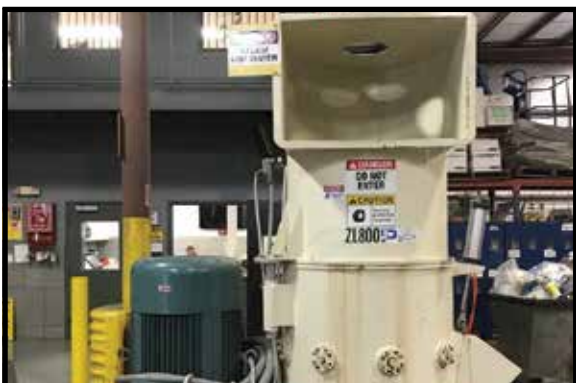
2014 ZL-800 PLASTIC & FILM DENSIFIER 177HP. 8 FIXED BLADES, 2 ROTARY. 600-800LBS/HR OF PP.
