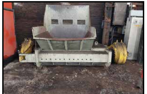
SHRED TECH ST500 HOOK SHEAR SHREDDER 2X 200 HP MOTORS. HOPPER AND VIBRATORY OUTFEED CONVEYOR
