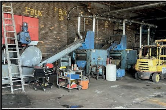
ELDAN TIRE RASPER SHREDDING LINE TAKES 2" CHIP DOWN TO 1/2" MINUS! READY TO START PROCESSING!
