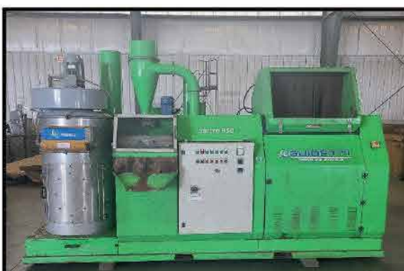
2011 GUIDETTI SINCR0 950 WIRE GRANULATOR PRODUCES 1,763 - 1,984 POUNDS PER HOUR
