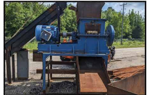
AMERICAN PULVERIZER MODEL 22 HAMMERMILL 100HP. 22" ROTOR. 3/4" SCREENS. FEED CONVEYOR. PRICE REDUCED!
