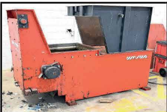
WEIMA WLK-4S SINGLE SHAFT SHREDDER DESIGNED FOR PLASTICS, WOOD, CARDBOARD.
