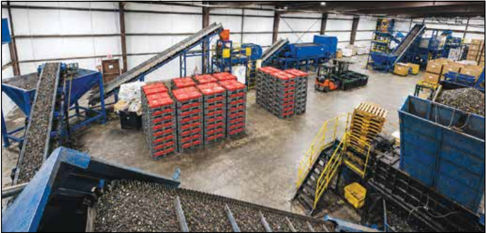
End-of-Life Vehicle (ELV) processing line going through size reduction, metal removal, density separation, and final electrostatic separation.
