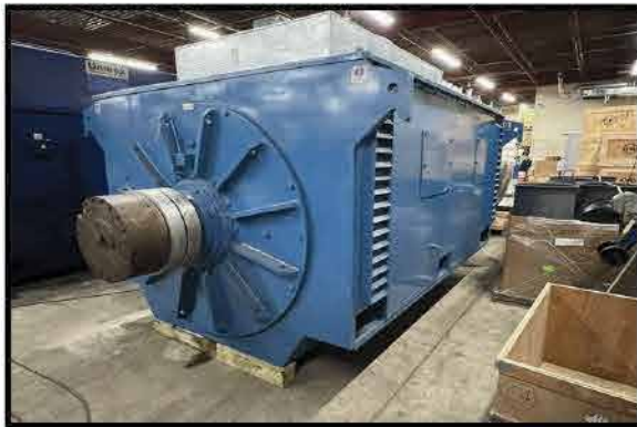
7,000 HP ALSTHOM SHREDDER MOTOR 4160 VOLTS, 446 RPM, 1068 AMP. TESTED GOOD IN 2024
