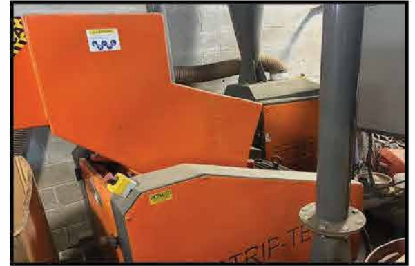
2012 STRIP-TEC MODEL 600 WIRE GRANULATOR 675 LBS/HR THROUGHPUT, 40 HP MILL
