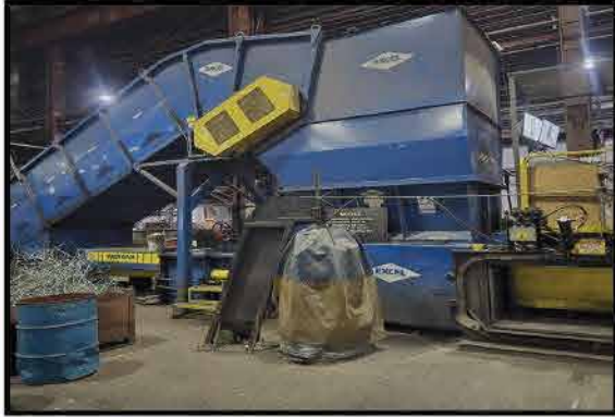
2008 EXCEL 2R10 TWO RAM METAL BALER PIT INFEED CONVEYOR IN GOOD CONDITION, CAN BE DEMONSTRATED
