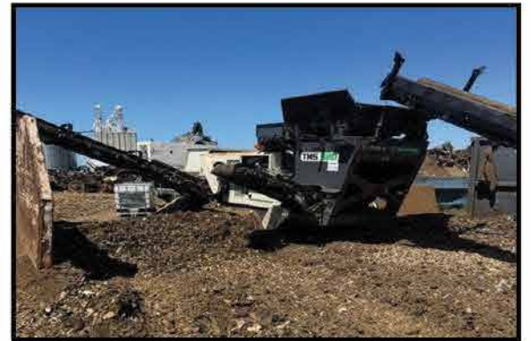
2024 TEREX/ECOTEC TMS320 METAL SEPARATOR SYSTEM INCLUDES 79" DRUM MAGNET AND EDDY CURRENT SEPARATOR.
