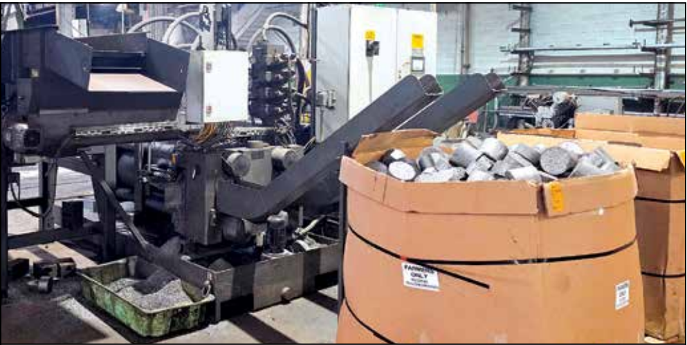
Innovative Recycling turns around 2,000 tons of steel turnings into puck-sized briquettes per month.
