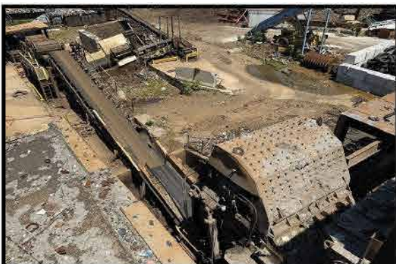
NEWELL 80X104 HAMMERMILL SHREDDER LINE 2,000 HP SCHORCH MOTOR. TONS OF SPARES INCLUDING A METSO BOX.
