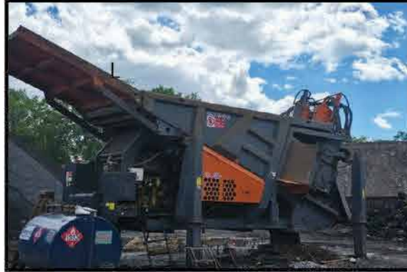
2023 BONFIGLIOLI SQUALO 2000 INCLINE SHEAR HOURS: 4,826, 6 CYLINDER CAT DIESEL ENGINE
