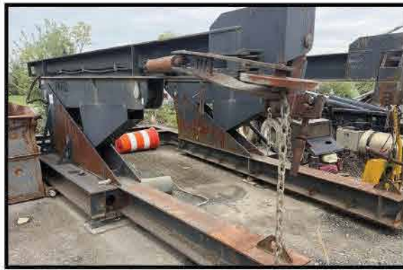
2007 A-WARD CONTAINER TILTER MODEL ACT 20 TILTS FROM -10 DEGREES TO 90 DEGREES, INCLUDES REMOTE CONTROL
