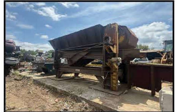
BEST 48 INCH VIBRATORY METERING BATCH FEEDER DIMENSIONS: HEIGHT 10', WIDTH 8', LENGTH 21.6'
