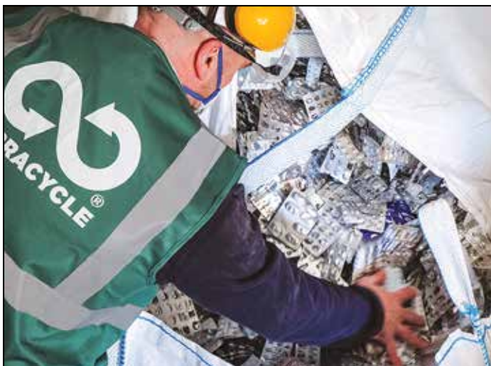
TerraCycle's incoming waste streams – such as the load of pill packaging seen here – are incredibly pure compared to those found at a material recovery facility.
