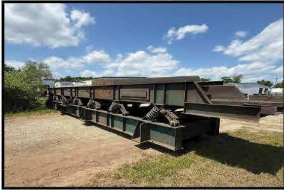
43' X 60" ACTION EQUIPMENT TAPER SLOT SCREENER 2" SCREENS INSTALLED, INCLUDES SET OF 1" SCREENS
