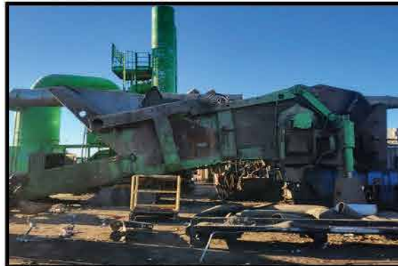
2020 BONFIGLIOLI DRAKE 16 HAMMERMILL 1,170HP MOTOR. FERROUS AND NON-FERROUS SEPARATION
