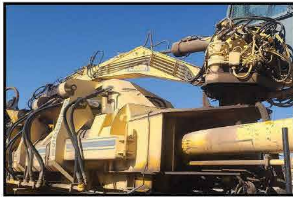
2006 COLMAR B 6200 SW AUTO LOGGER/BALER PRODUCES 34" X 25" VARIABLE-LENGTH LOGS/BALES
