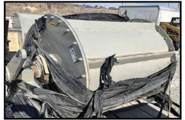
2011 ERIEZ 48"X48" DRUM MAGNET NEVER PUT INTO SERVICE! APPROX. 1,600 GAUSS AT DRUM SURFACE
