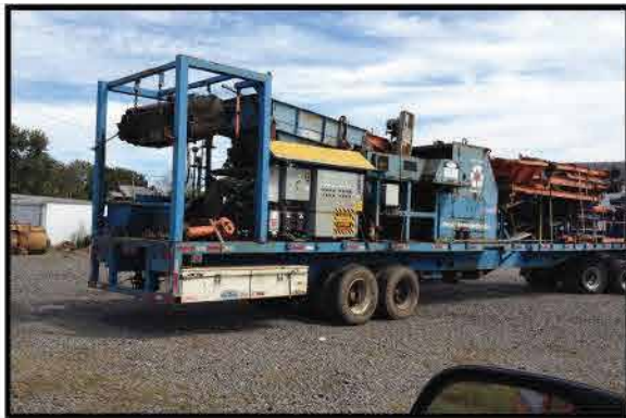
HOAT METALS REMEDIATION SYSTEM PORTABLE TROMMEL AND EDDY CURRENT SYSTEM
